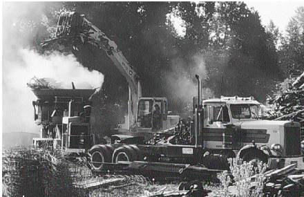
Figure 27: wood waste at chipping facility (top) and Figure 28: demolition debris being chipped on-site (above) (KPG, Inc.)
