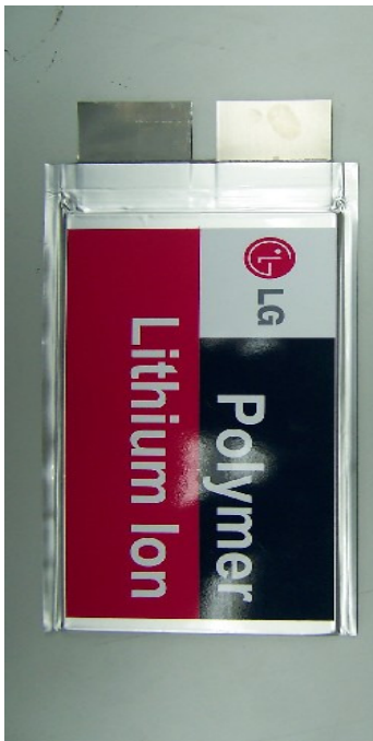
Fig. 4. Picture of an HEV Cell using Al-polymer laminate packaging.
