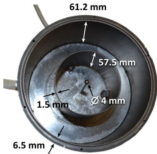
Figure 3. Disassembled NE2575. When irradiating the chamber, the central electrode should be pointed directly towards the source. The thickness of the rear wall (not shown) is 1.5 cm. The outer cylindrical radius of the chamber is 6.255 cm.
