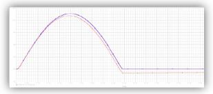
These seemingly small amplitude deviations can result in significant errors during numerical integration<sup>1</sup>. A DC-response device has no such problem because it can follow the slow-moving input accurately. In real day-to-day applications, physical inputs do not resemble half-sine impulses, but the basic problem remains whenever one needs to track slow motion with an ac coupled device.
