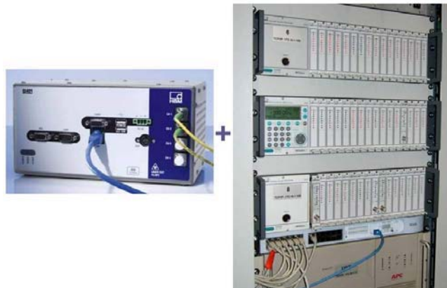
Fig. 13: SI-405 optical interrogator together with MGCplus
