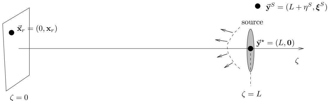
Figure 1: Setup for imaging a distributed source with a planar array of transducers
