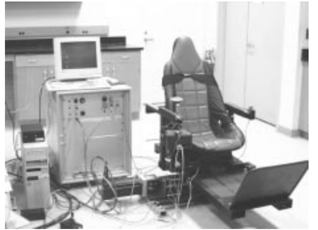
Figure 4. The Experimental Apparatus, showing the host computer, electronic cabinet, and motion platform with joystick
