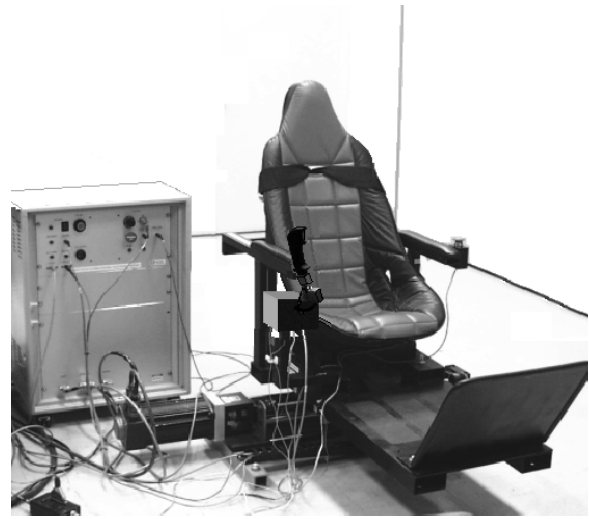
Fig. 6. The single-axis motion platform is driven by DC motor and ballscrew and features a joystick accessible to the right hand of a seated operator.
