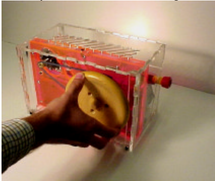
Figure 4. The finished Plexiglas Box. The emergency stop button is visible on the right and the cable drive is visible inside the clear housing.
