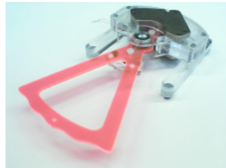
Figure 1. The iTouch motor. A user generally rests his or her wrist on the housing/magnet assembly and extends their fingers to rest on the end of the crescent-shaped handle.
