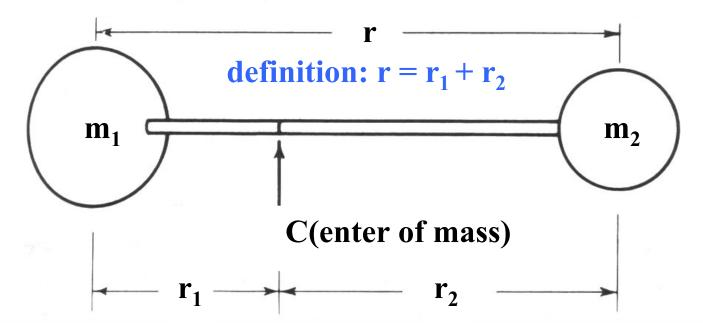
Balancing equation:  $m_1r_1 = m_2r_2$
