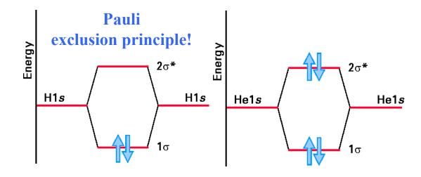
$H_2$ :  $1\sigma^2$ "He<sub>2</sub>":  $1\sigma^2 2\sigma^{*2}$ More strongly and closely bonded than H<sub>2</sub><sup>+</sup>
