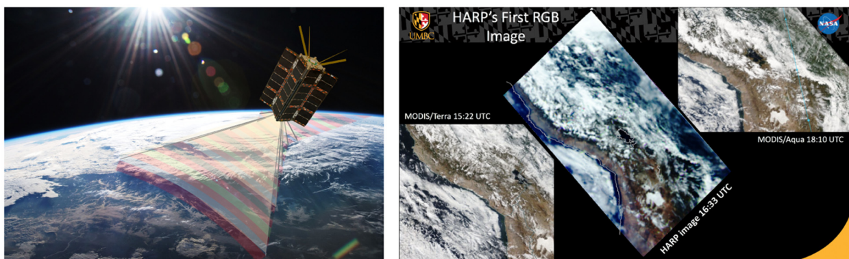
FIGURE 4.7 HARP wide field-of-view imaging polarimeter CubeSat flight validation mission demonstrating multi-angle aerosol and cloud property measurements from space. This technology was matured from an airborne system into a space-borne version where a long data capture of 400 images over Lake Titicaca in South America were post-processed into a pushbroom image. Similar images taken by the Moderate Resolution Imaging Spectroradiometer (MODIS) instrument on the Aqua and Terra satellites are also shown confirming the atmospheric and land features seen in the HARP data. Lake Titicaca serves as an excellent clean air vicarious calibration source for this polarimetric imager given the lake's high altitude providing excellent visibility of the sun's reflection off the surface and polarization from to the atmosphere. SOURCE: HARP Team, University of Maryland Baltimore County. https://esi.umbc.edu/hyper-angular-rainbow-polarimeter/ .
