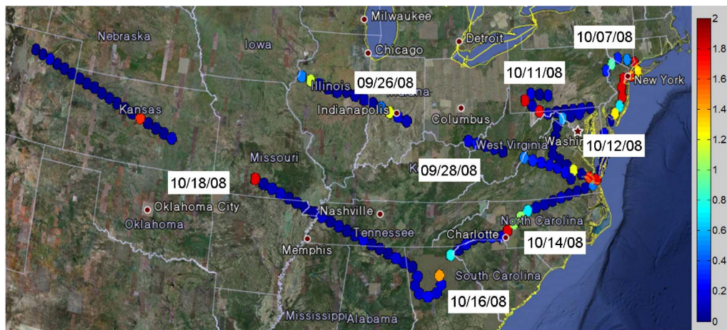
Fig. 1. SMAPVEX08 flight paths utilized in RFI analysis (excluding 10/6/08 data). Geolocated RFI brightness temperatures at a spatial resolution of 40 km and with H polarization (colorscale in kelvin). From [19] with permission from the author.
