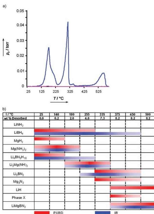
**Figure 4.** a) TPD-MS data for the ternary composition depicting hydrogen ( $m/z$  2, blue) and ammonia ( $m/z$  17, pink) as a function of temperature (heating at 5 °C min<sup>-1</sup> to 575 °C). b) Phase composition as a function of desorbed hydrogen amount (wt%) and temperature (°C) as determined from the static PXRD and IR data.
