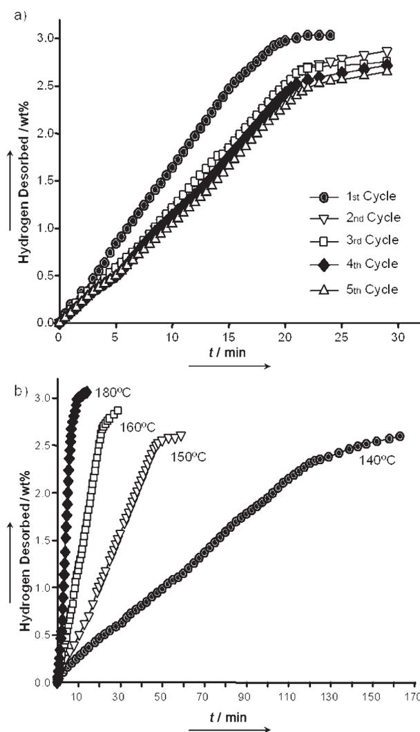
**Figure 2.** a) Hydrogen desorption kinetics at  $160^\circ\text{C}$  and 1 bar over five cycles after subsequent charging ( $160^\circ\text{C}$  and 100 bar hydrogen). b) Reversible isothermal kinetic hydrogen desorption data (to 1 bar) for the ternary composition based on the second desorption cycle at  $140^\circ\text{C}$  (●),  $150^\circ\text{C}$  (▼),  $160^\circ\text{C}$  (□), and  $180^\circ\text{C}$  (◆) versus time.
