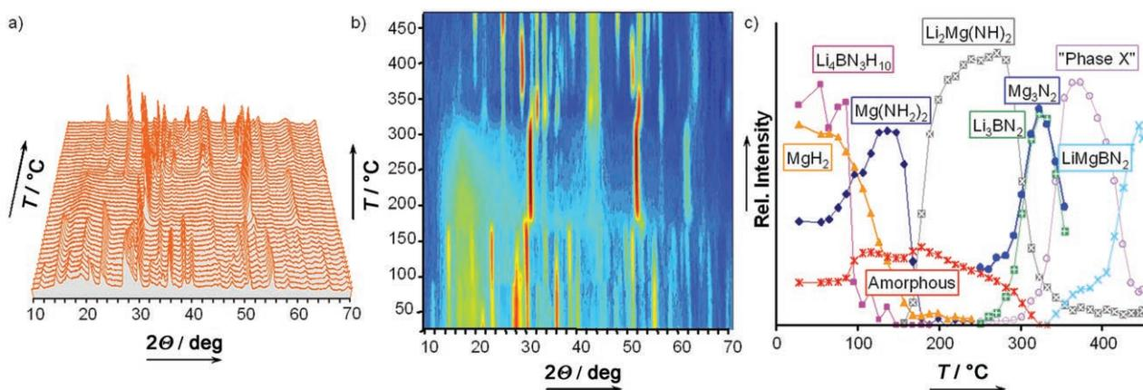
**Figure 5.** a) Raw PXRD data for the ternary composition as a function of temperature ( $25$ – $450^\circ\text{C}$ ). b) The corresponding two-dimensional contour plot derived from the raw patterns in (a). c) Plot of the relative amounts of individual phases as a function of temperature.
