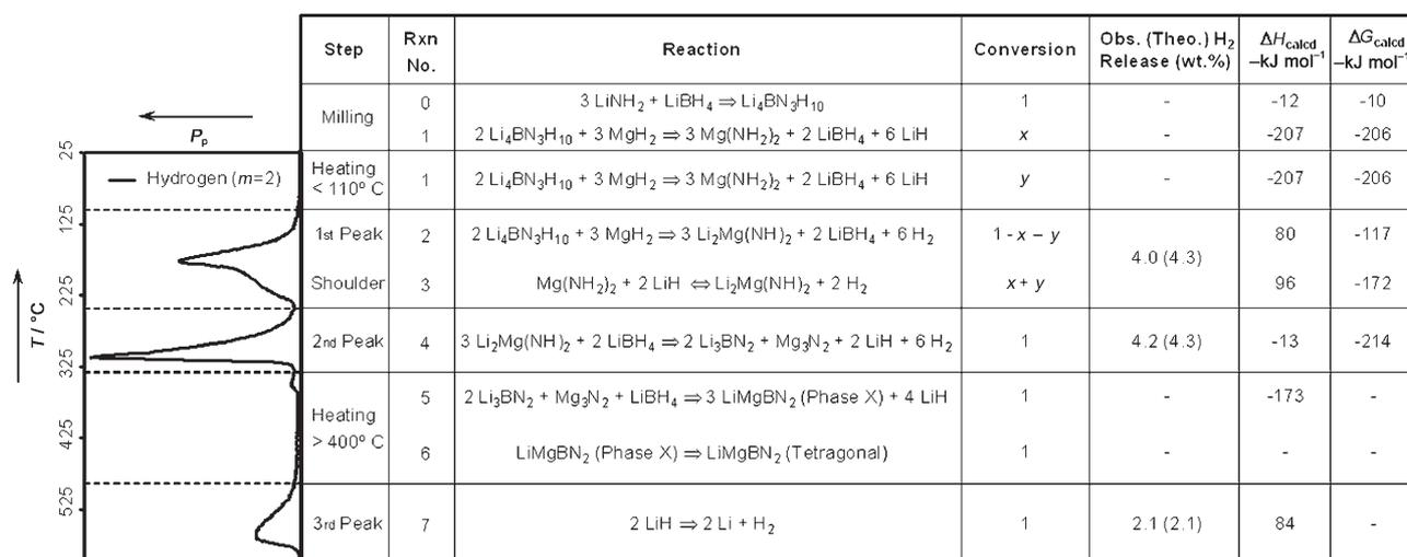
**Figure 6.** Proposed reaction pathway for the ternary composite, including the observed/theoretical hydrogen capacity, reaction enthalpy ( $\Delta H$ ), free energy ( $\Delta G$ ) (both in  $\text{kJ mol}^{-1}$  for products at 300 K), and the corresponding temperature range (coupled to the TPD-MS curve). The reaction numbers in this figure correspond to those used in the text.
