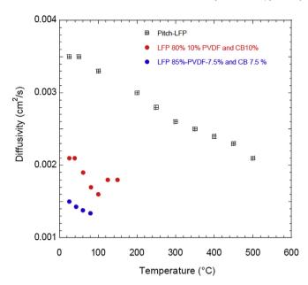
**Fig. 5.** Thermal diffusivity versus temperature of LiFePO<sub>4</sub> + pitch (box) and 10 and 7.5 wt.% PVDF composition (red and blue circles). (For interpretation of the references to colour in this figure legend, the reader is referred to the web version of this article.)
