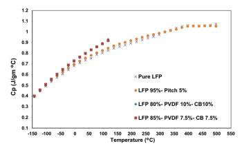
**Fig. 3.** Heat capacity versus temperature of LiFePO<sub>4</sub> (cross) from Hydro-Québec, LiFePO<sub>4</sub> + pitch (solid circle) and LiFePO<sub>4</sub> + PVDF + carbon black (solid squares and diamond). The binder compositions are limited to 120 °C due to the low melting point of PVDF.
