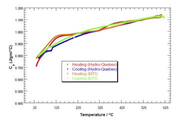
**Fig. 2.** Heat capacity versus temperature (between 25 and  $600\,^{\circ}$ C) of LiFePO<sub>4</sub> obtained from two suppliers, Hydro-Québec and MTI respectively. Data are shown for both heating and cooling cycle. The sample from Hydro-Québec has between 2 and 3 wt.% carbon content.
