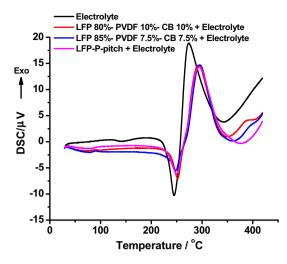
**Fig. 6.** DSC result of LFP electrode compositions with electrolyte mixture (1.2 M LiPF $_6$  + EC + DMC). Black line: electrolyte mixture only. Blue line: LFP electrode composition, 80% LFP + 10% C-black + 10% PVDF. Green line 85% LFP + 7.5% C-black + 7.5% PVDF. Red line: LFP + 5 wt.% coated pitch only. (For interpretation of the references to colour in this figure legend, the reader is referred to the web version of this article.)
