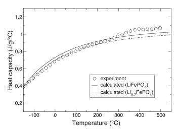
**Fig. 4.** Calculated heat capacity using DFT and comparison with experimental data for Hydro-Québec LFP as a function of temperature. Solid line shows the calculated heat capacity of pure LiFePO<sub>4</sub>, while the dashed line shows that of a two-phase mixture of 70 mol % LiFePO<sub>4</sub> and 30 mol % FePO<sub>4</sub>.
