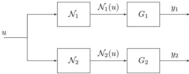
Fig. 1. SIMO Hammerstein system,  $\mathcal{N}_1$  and  $\mathcal{N}_2$  represent memoryless nonlinearities, and  $y_1$  and  $y_2$  represent outputs of the linear transfer functions  $G_1$  and  $G_2$ , respectively.
