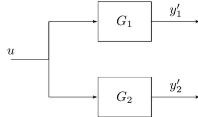
Fig. 3.  $y'_1$  and  $y'_2$  are the outputs of the linear transfer functions  $G_1$  and  $G_2$ , respectively, with input  $u$ . This system does not exist and is used only for analysis
