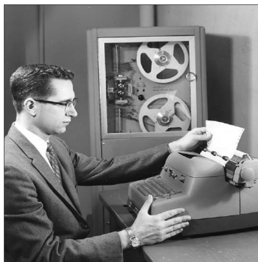
Graduate student Stanley C. Jones using the Ford Foundation Project Bendix G-15 computer to solve reservoir engineering problems involving unsteady-state flow of water in porous beds.
