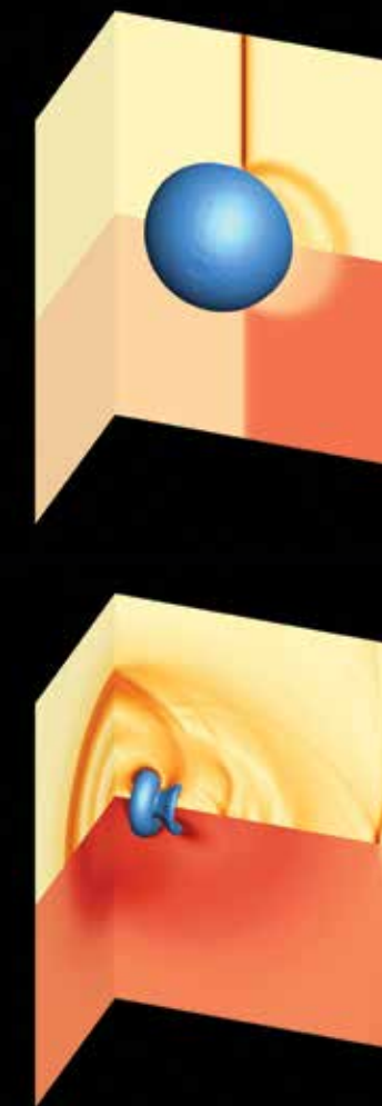
ABOVE: Shock-induced collapse of a bubble near a rigid surface. The incoming shock wave (moving right to left) in water interacts with a preexisting gas bubble and causes its collapse. High pressures and temperatures are achieved during this process, leading to potential structural damage to the neighboring solid (on the left side). This mechanism is thought to play a critical role in cavitation erosion to propellers, in high-intensity focused ultrasound and in certain traumatic brain injuries.
