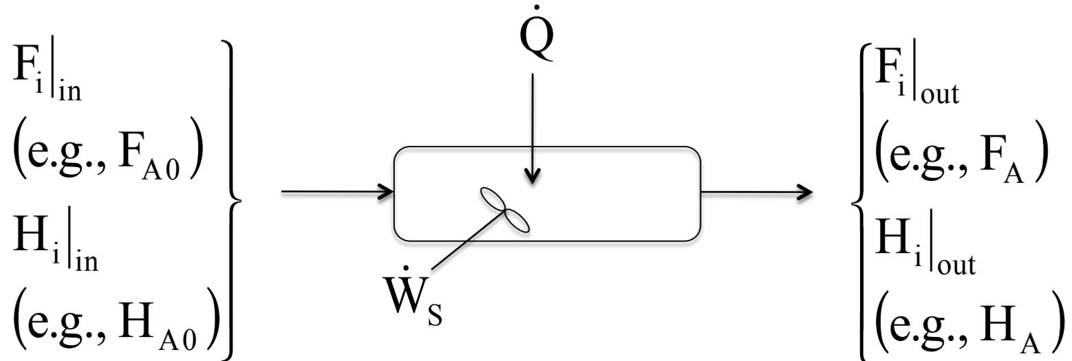
*Energy Balance on an open system: schematic.*
