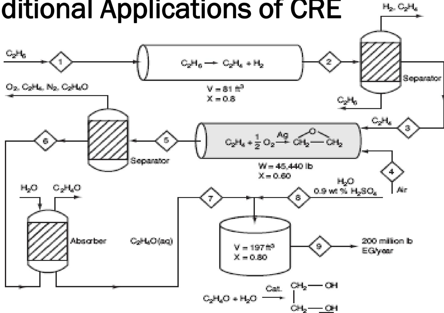
Chemical Plant for Ethylene Glycol (Ch. 5)
