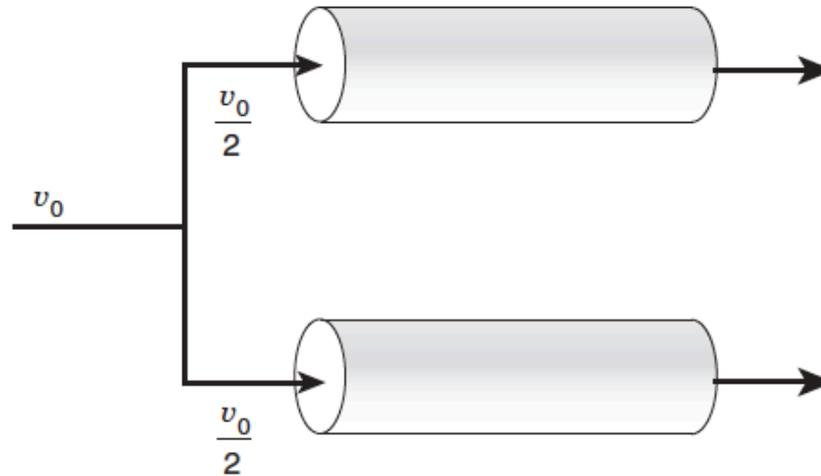
Figure E14-4.2 Parallel arrangement.
