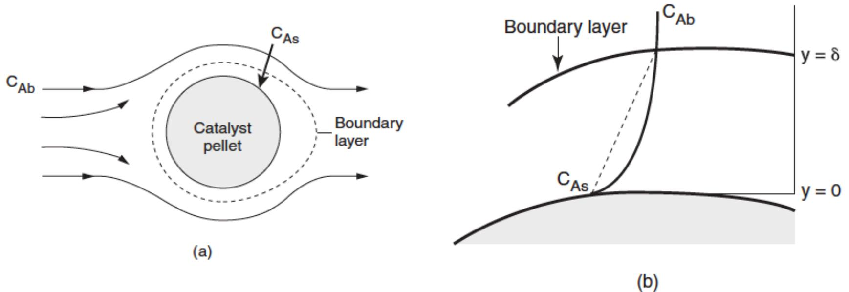
**Figure 14-1** Boundary layer around the surface of a catalyst pellet.
