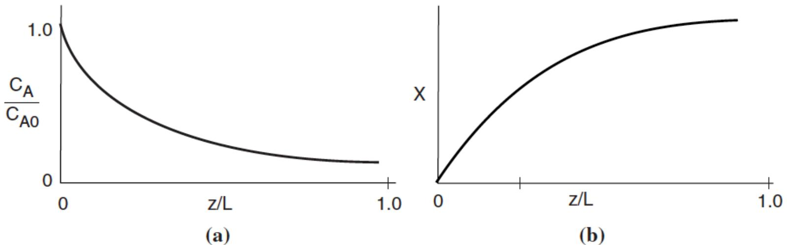
**Figure 14-7** Axial concentration (a) and conversion (b) profiles in a packed bed.
