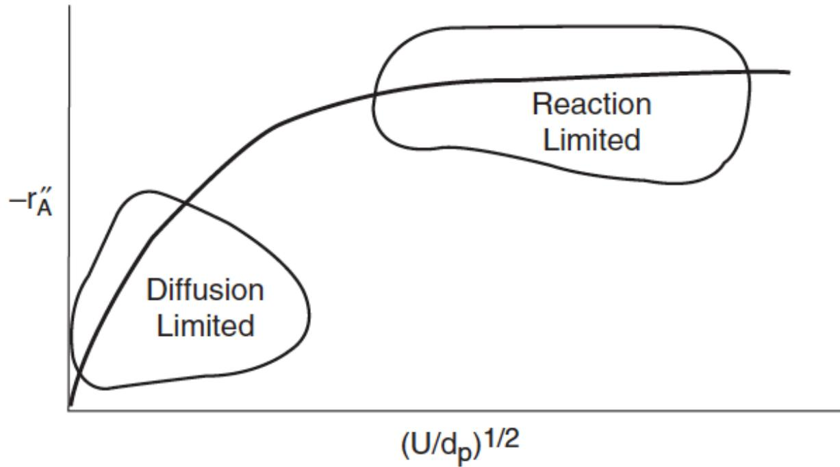
**Figure 14-4** Regions of mass transfer–limited and reaction–limited reactions.
