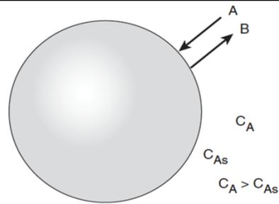
Figure 14-3 Diffusion to, and reaction on, external surface of pellet.
