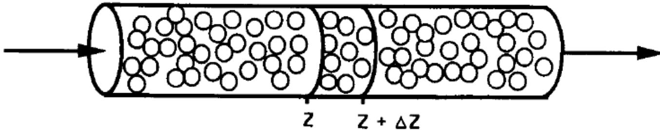
Figure 14-5 Packed-bed reactor.
