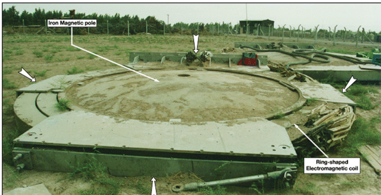
Figure 19. Photograph of Iraqi EMIS electromagnet.
