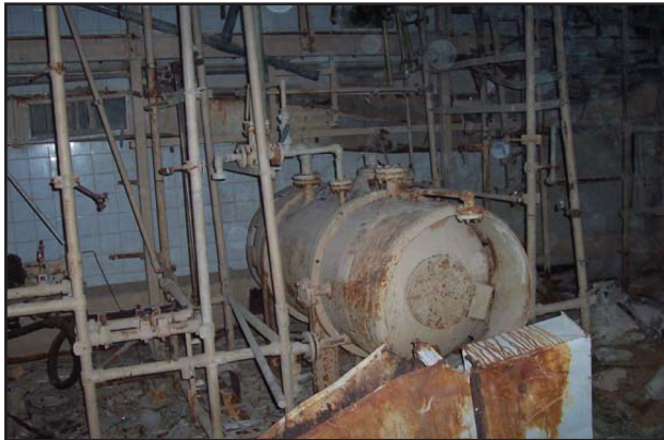
Figure 3. A two ton bulk storage cylinder found in the underground pilot plant at Al Muthanna. The storage container had been modified in the 1980s into a reactor vessel probably for mustard production. This item escaped UNSCOM-directed destruction.
