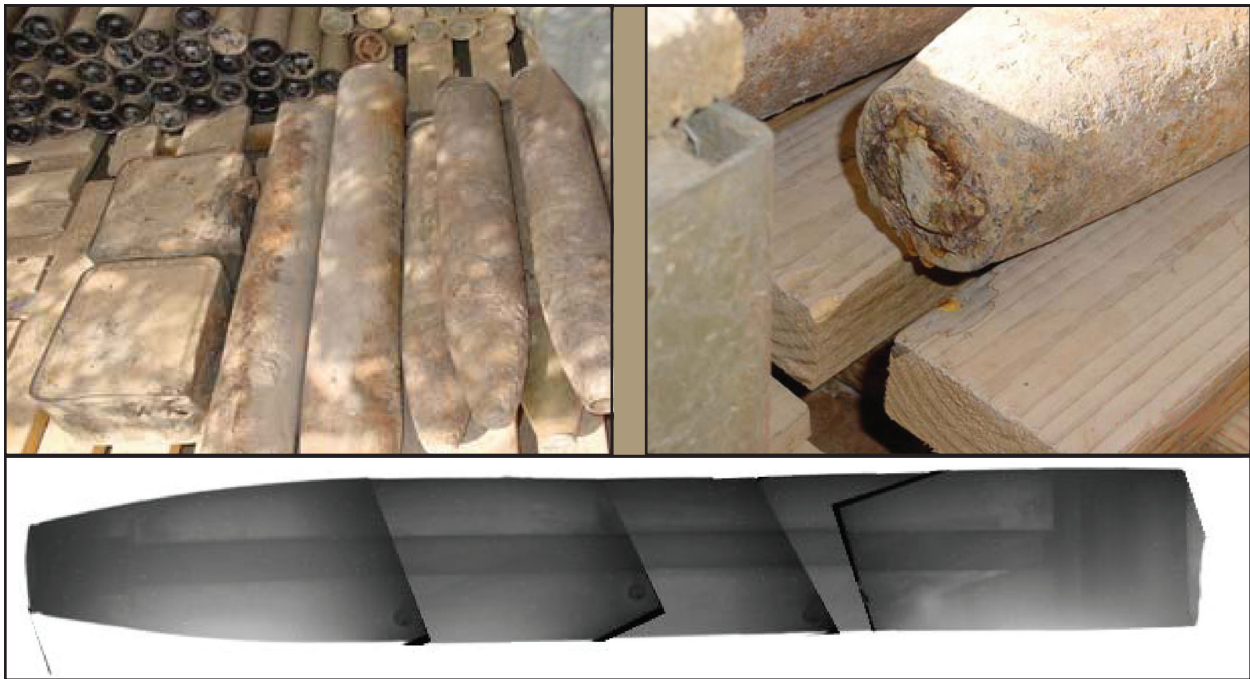
Figure 7. Photos and x-ray of SAKR-18 rockets.
