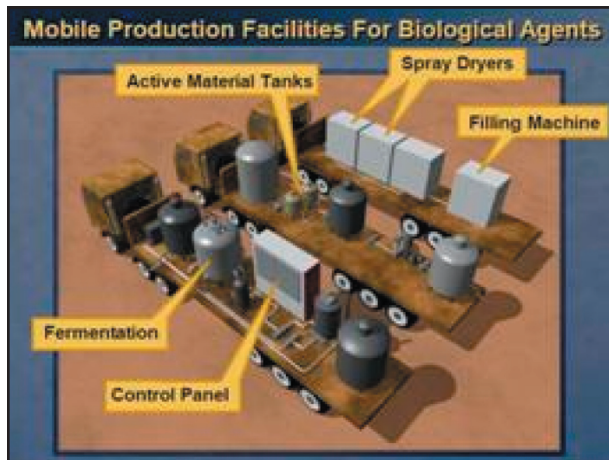
Figure 11. Truck-mounted BW production unit-based on source reporting.
