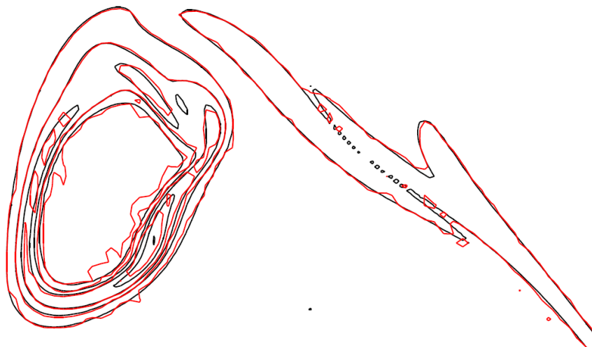
Figure 14. Iso-contours of the dimensionless vorticity norm, \frac{L}{V_0} |\omega| = 1, 5, 10, 20, 30 , on a subset of the periodic face \frac{x}{L} = -\pi at time \frac{t}{t_c} = 8 . Comparison between the results obtained using the pseudo-spectral code (black) and those obtained using a DG code with p = 3 and on a 96^3 mesh (red).
