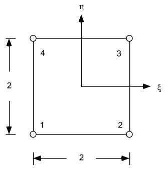
We shall make an analysis of finite element interpolation error of the 4 node quadrilateral element for plane problems using Taylor's exansion of an arbitrary function g in *Mathematica*:
