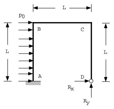
The frame structure consists of three beams, the length of which is the same, say L. At point A, it is fixed, i.e., the deflection and rotation ( the slope of the deflection ) are constrained to be zero, while it is supported by a hinge at D. A uniformly distributed load,  $p_0$ , is applied along the
