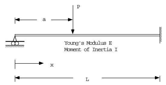
If the reaction at the hinge support is denoted by Ra, the bending moment distribution becomes
