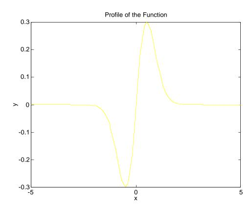
Since the given function is anti-symmetric at x=0, the value of interal must be zero. Applying the extended trapezoid rule, we have
