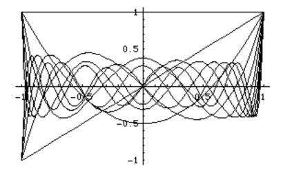
Legendre polynomials  $P_n(x)$ , n = 0,1,2,...., are obtained by the orthogonalization of the polynomial basis functions  $\{1, x, x^2,.....\}$  with respect to the inner product
