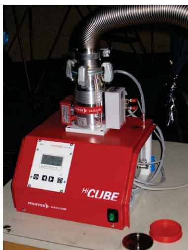
(a) Vacuum pump with hose attached. The power switch is the green switch in the lower-right. The right-most button near the display is the turbo-pump on/off switch. The blank-off and cap are in the lower-right.
