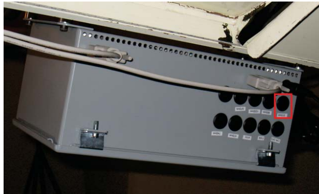
(c) Control box; the 810nm on/off switch is marked in red
