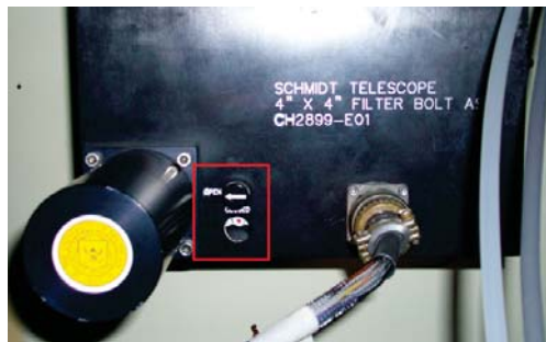
Figure 6: The filter status hole on the filter changer mechanism.
