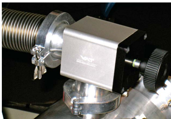
(b) Pressure valve on the camera with hose attached. The valve is the black knob on the right
