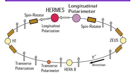
Self polarization of electrons by Synchrotron radiation emission in curved sections:
