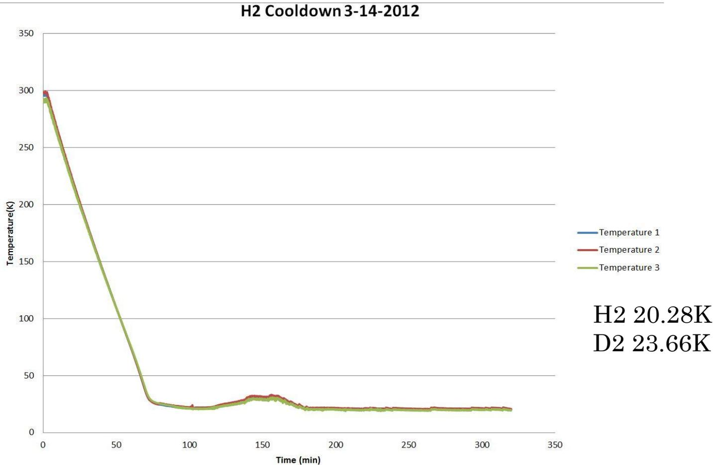
The cooldown takes less than an hour. But the actual fill during the experiment took 16h for H<sub>2</sub> and 12h for D<sub>2</sub>.
