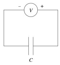
Starting with an uncharged capacitor and zero voltage, we isothermally increase the voltage, so as to charge the capacitor.
