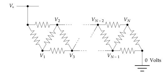
All the resistors have the same resistance R. The power rail at the top is at voltage  $V_+ = 5$ V. The problem is to find the voltages  $V_1 \dots V_N$  at the internal points in the circuit.
