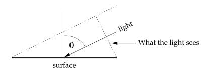
So the intensity of illumination is  $a \cos \theta$ , if a is the raw intensity of the light. This simple physical law is a central element of 3D computer graphics. It allows us to calculate how light falls on three-dimensional objects and hence how they will look when illuminated from various angles.
