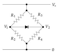
The resistors obey the normal Ohm law, but the diode obeys the diode equation:
