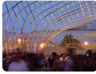
Canopy, created by nArchitects, was a temporary environment constructed of weather integrated bamboo. The bamboo structure provided shade as well as mist and fog built into the bamboo.
