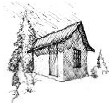
Figure 46: Sketch of proposed reconstructed sauna using straw bales for a loadbearing wall and reusing rough-sawn cedar and roof rafters
