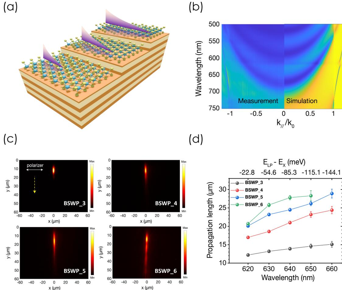
**Figure:** (a) Schematic of polariton systems comprising WS<sub>2</sub> monolayers and distributed Bragg reflectors (DBR). (b) Measured and simulated angular reflectivity spectra of a polariton structure (BSWP-5). (c) Structure-dependent polariton propagation. (d) Comparison of wavelength-dependent propagation lengths for different samples.
