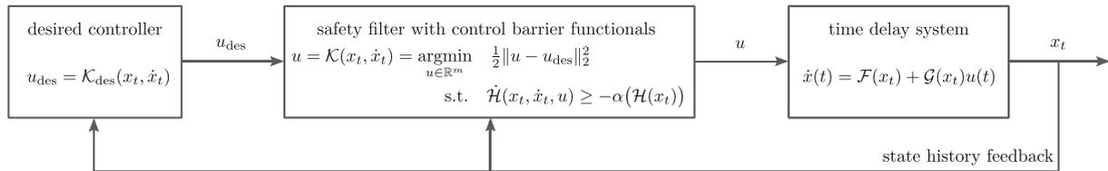
**FIGURE 1** Block diagram of the proposed control framework that provides formal safety guarantees for the control loops of time delay systems. A safety filter, that is established based on the proposed *control barrier functionals*, is applied to modify a nominal (not necessarily safe) control input and guarantee safe behavior for time delay systems through state history feedback.
