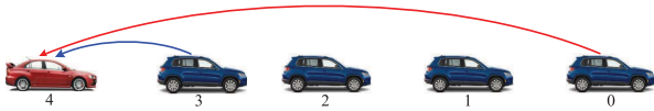
Fig. 4. A vehicle network where the CCC vehicle 4 monitors the motion of vehicle 3 via range sensors and also receives information from vehicle 0 by V2V communication.
