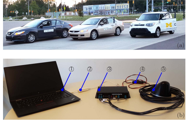
Fig. 11. (a) Two human-driven vehicles and one connected automated vehicle used in the experiments. The two vehicles on the left are only equipped with V2V communication devices, while the vehicle on the right is capable of automated driving as well as V2V communication. (b) The V2V communication on-board unit: ① upper-level computer, ② ethernet cable, ③ electronic control unit, ④ power cable, ⑤ V2V/GPS antennae.
