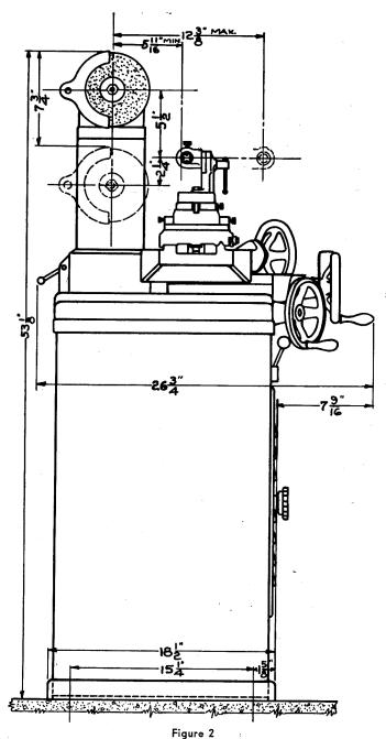
Keep back of base about 8 inches away from nearest wall to allow for swivel of wheel head.
