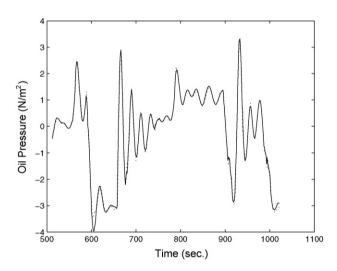
**Fig. 6.** Identification of hydraulic robot arm dynamics by non-Mercer hybrid kernel LP-SVR on the validation set (solid line: observation, dotted line: model from hybrid kernel LP-SVR).
