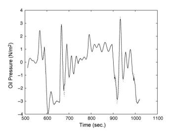
**Fig. 4.** Identification of hydraulic robot arm dynamics by GRBF kernel QP-SVR on the validation set (solid line: observation, dotted line: model from GRBF kernel QP-SVR).
