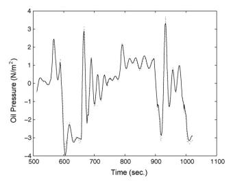
**Fig. 2.** Identification of hydraulic robot arm dynamics by GRBF kernel LP-SVR on the validation set (solid line: observation, dotted line: model from GRBF kernel LP-SVR).
