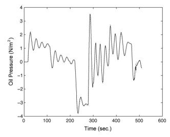
**Fig. 5.** Identification of hydraulic robot arm dynamics by non-Mercer hybrid kernel LP-SVR on the training set (solid line: observation, dotted line: model from hybrid kernel LP-SVR).
