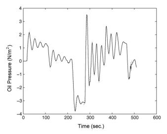
Fig. 1. Identification of hydraulic robot arm dynamics by GRBF kernel LP-SVR on the training set (solid line: observation, dotted line: model from GRBF kernel LP-SVR).
