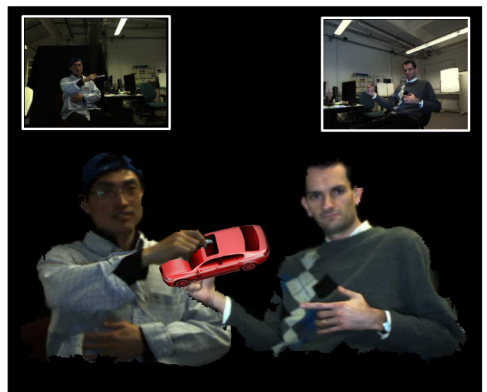
Fig. 1. Two users interacting with a virtual car model each captured with a different stereo camera and rendered inside a shared virtual environment using the stereo vision system presented in this paper.
