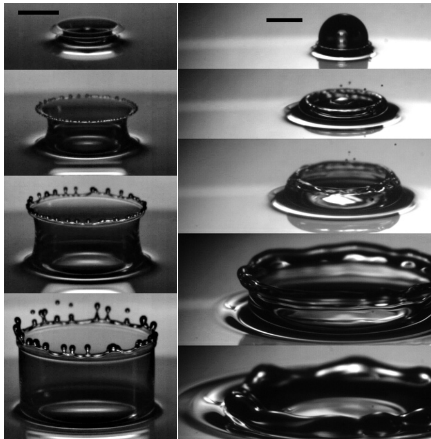
Figure 10. Left: Crown splash without a microdroplet splash. Silicon oil, Re = 966 , We = 874 , H = 0.2 at 200, 740, 1410, 2430 \mu s after impact. Corresponds to \blacktriangledown in Fig. 3. Right: Microdroplet splash without a crown splash. Glycerol/water mixture Re=1910 , We=142 , H = 0.2 at 260, 940, 1780, 6880, 11200 \mu s after impact. Corresponds to \blacktriangle in Fig. 3. Scale bar corresponds to 2 mm.
