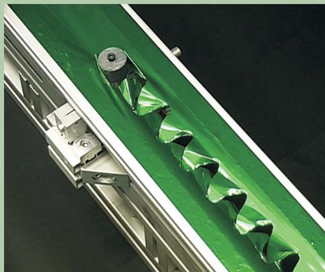
Figure 4. A wavy crack pattern is created by dragging a blunt cutting tool through a thin plastic sheet gripped along its sides. 10 (Courtesy of Benoît Roman.)
