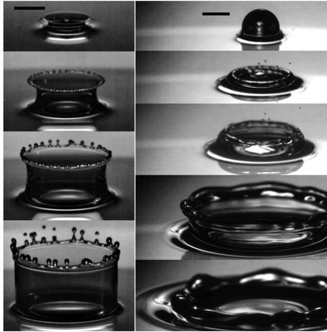
Figure 10. Left: crown splash without a microdroplet splash. Silicon oil, Re = 966 , We = 874 , H = 0.2 at 200, 740, 1410, 2430 \mu s after impact. Corresponds to \blacktriangledown in figure 3. Right: microdroplet splash without a crown splash. Glycerol/water mixture, Re = 1910 , We = 142 , H = 0.2 at 260, 940, 1780, 6880, 11200 \mu s after impact. Corresponds to \blacktriangle in figure 3. Scale bar corresponds to 2 mm.
