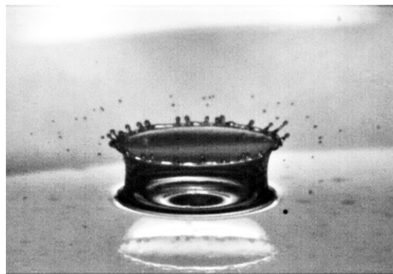
Figure 7. An ejecta sheet ‘riding’ on a Peregrine sheet. The former leads to the formation of tiny droplets that precede the much larger Peregrine sheet. Re = 1354 , We = 874 , 580 \mu s after impact. Corresponds to ★ in figure 3.
