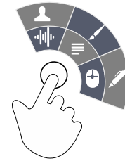
Figure 12: An illustration of a custom contextual pie menu for touchscreen devices. We created three implementations with minimal changes to the gesture's implementation: 1) the user holds their finger then selects a menu item, 2) the user taps their finger then selects a menu item, or 3) the user double taps their finger then selects a menu item.
