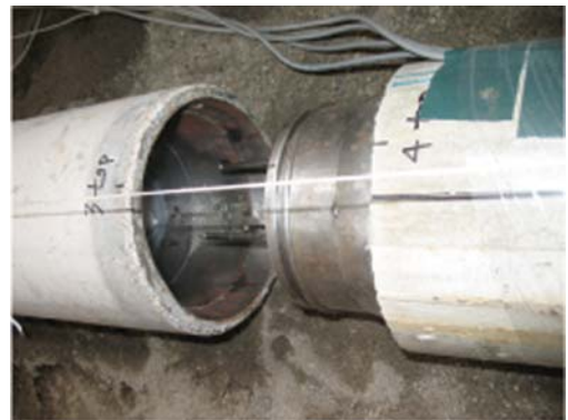
Figure 2. Typical bell-and-spigot connection between two pipe segments. The three potentiometers shown inside the pipe were used to measure displacement and rotation at the joint.
