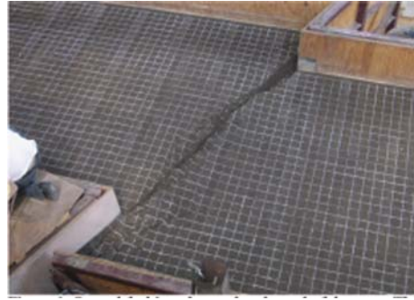
Figure 6. Ground faulting observed at the end of the test. The gridlines shown are spaced at approximately 10 \text{ cm} .
