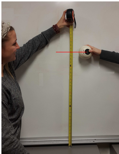
Figure 8: The g ball experiment. Note that measurements are done at the ball's center (red line).
