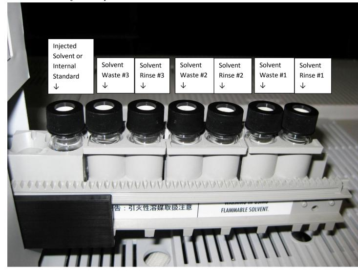
The vials in the injector tray are 4 ml autosampler vials with a Teflon-lined cap, such as Fisher Scientific part # 03-391-22.
