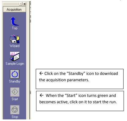
7) When the data acquisition is complete, click on "Top" icon on the left hand side to move up one level. Then, click on the "Data Analysis" icon.
