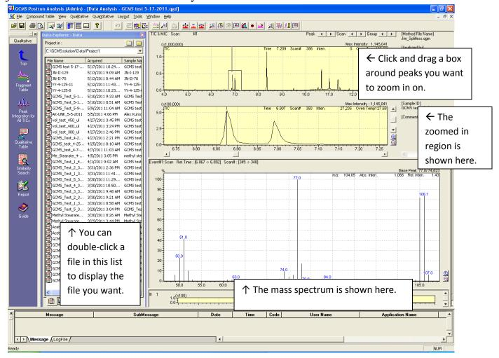
To display a mass spectrum of a chromatographic peak: right-click the mouse anywhere in the chromatogram to obtain a menu. Then left-click on "Average Spectrum" to get a cursor. Left-click and drag the cursor across the chromatographic peak, and its mass spectrum will be displayed.
