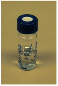
The minimum volume of solution is 450 ul. If you cannot spare that much solution, you can use a conical glass insert in the vial, so that the solution level will be high enough for the syringe needle to enter it.
